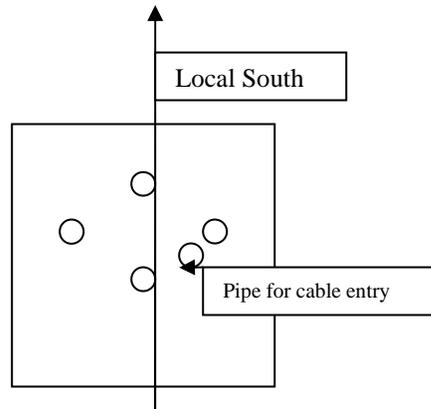
Mark the position of the foundation as shown to point one axis to the Geographical south-locate and mark the Local south Direction by locating the Pole star (Dhruva Tara). Adjust the center to center distance 500 mm between bolt centers, while ensuring a cover of at least 50 mm is available to the bolts-tied to the re-bar. Embed a pipe approx 2 inch dia for taking cables below ground level to the controller.
